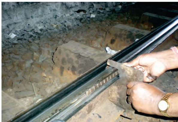
Fig. 2.8 : Measurement of wear on outer rail
