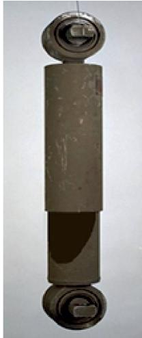
Normal contamination caused by the operating environment of the dampers is harmless.
