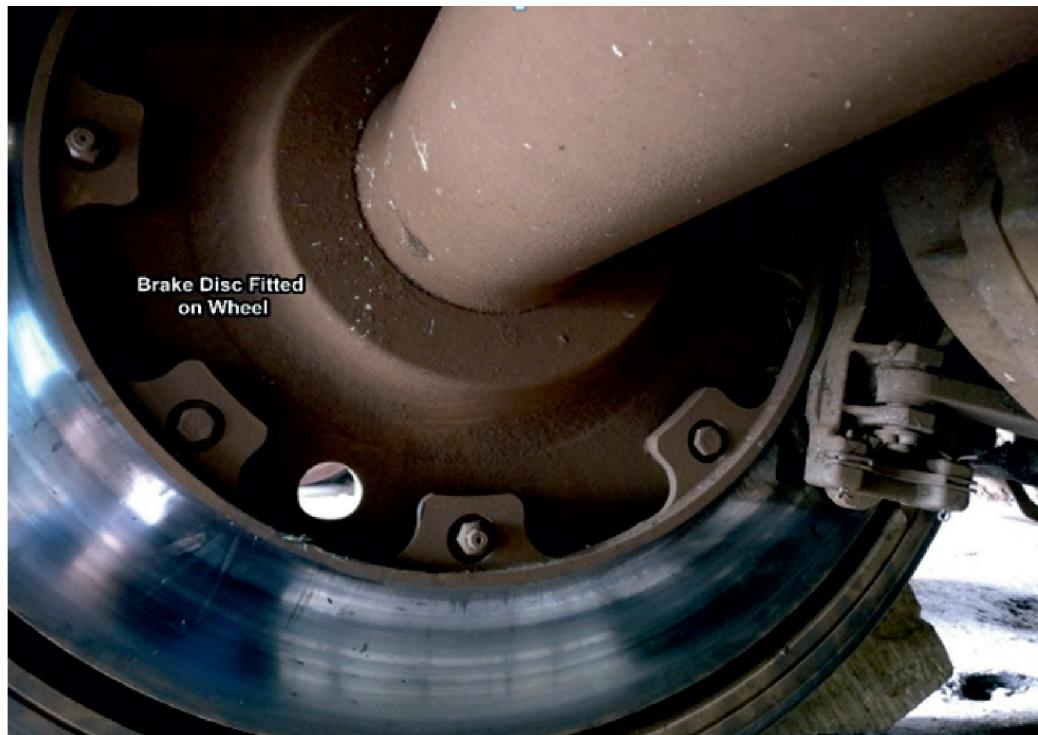
**Fig 9 : Wheel assembly showing fitment of brake disc**
