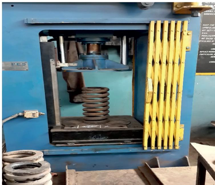
**Fig 38 : Spring deflection testing machine**
