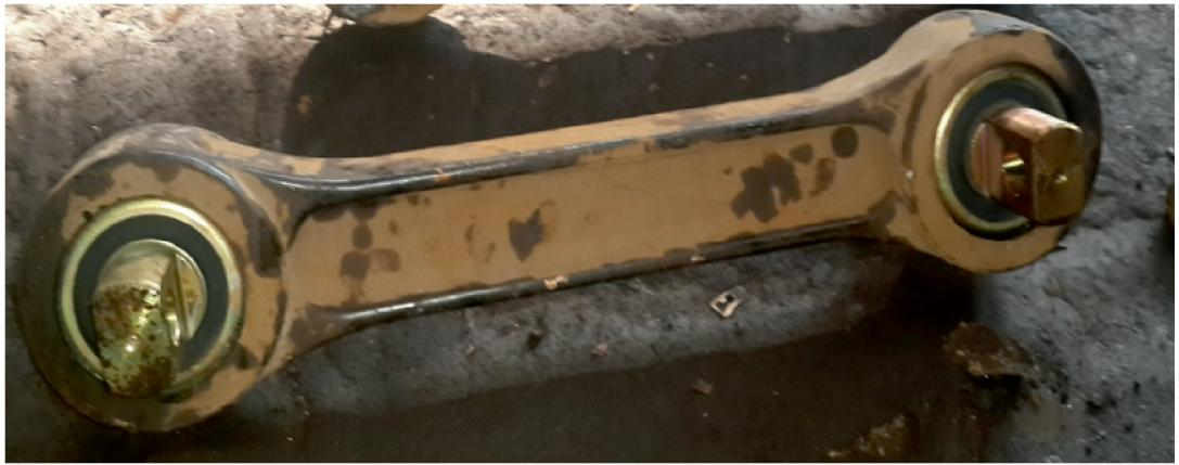
**Fig 57 : Photo of Guide rod with spheriblocs**
