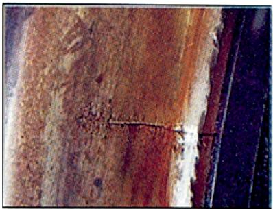
**Fig: 32 Thermal crack on tread**
