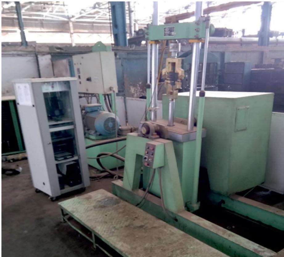
**Fig 50 : Hydraulic damper testing machine**
