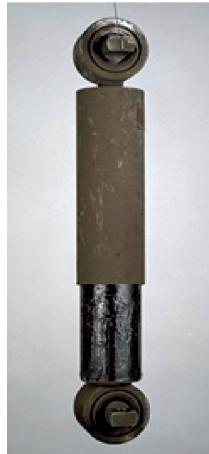
A strong oil leakage becomes apparent by a damp surface, which usually covers a large part of the reservoir tube.
