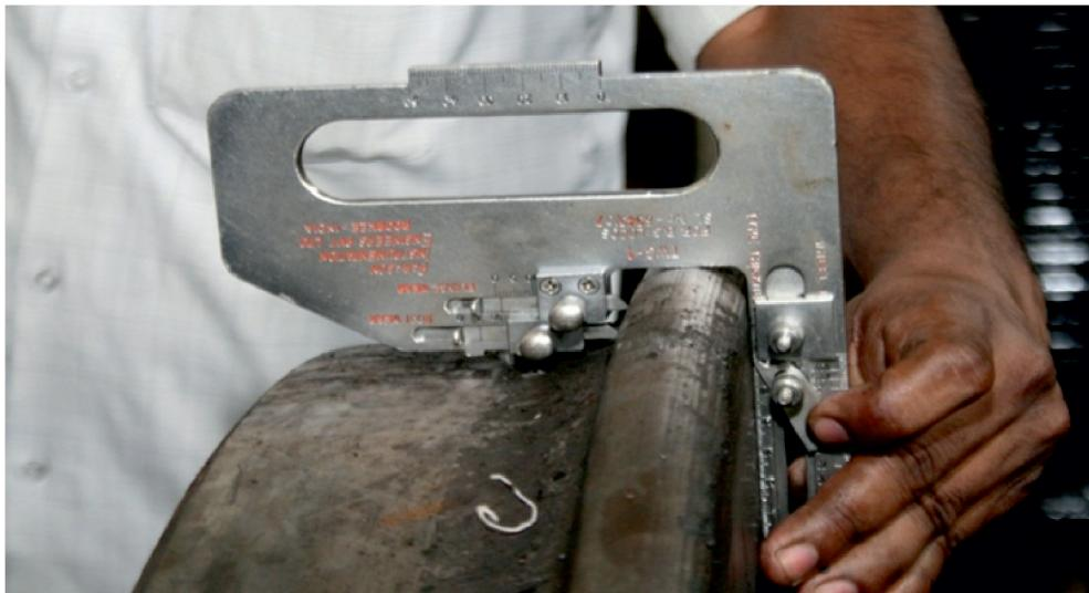
**Fig 23 : Procedure for checking wheel root wear**
