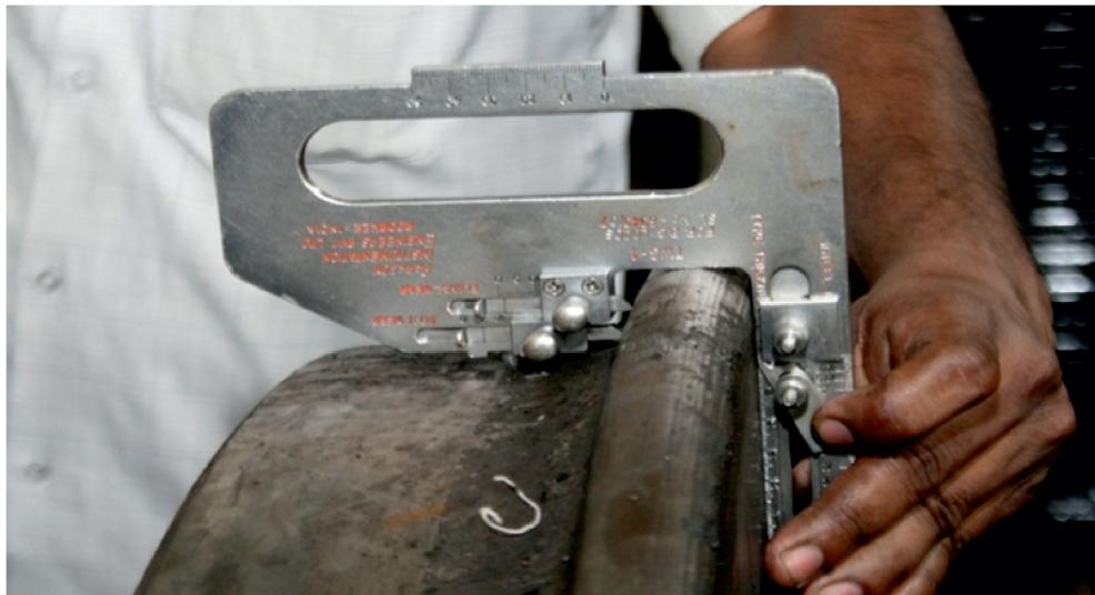
**Fig 21 : Procedure for checking wheel flange wear**
