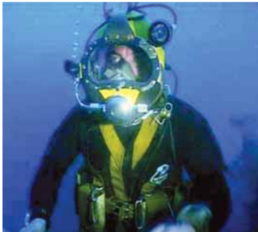
Fig. 3.2 Surface supplied air diving
