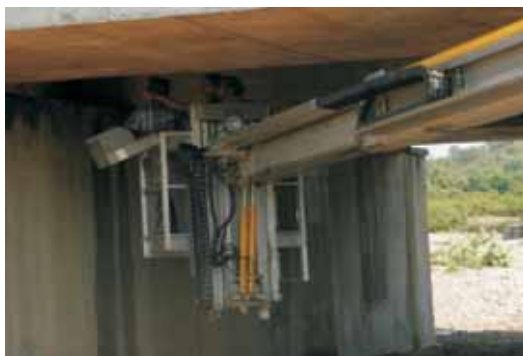
Fig 1.10: Bucket of MBIU is lowered under bridge
