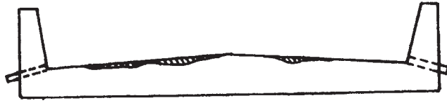
Fig. 2.42 Formation of depressions due to absence of wearing coat
