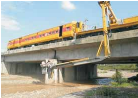
Fig 1.9: Power pack and inspection vehicle with lowered arm of MBIU
