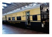
of TRCs are computerized TRCs, and uses inertial principle of obtaining vertical and lateral profile of individual rails. These TRCs have capability to generate reports of Track Geometry parameters on two user selectable Chord in the range of 2 to 20 m.
